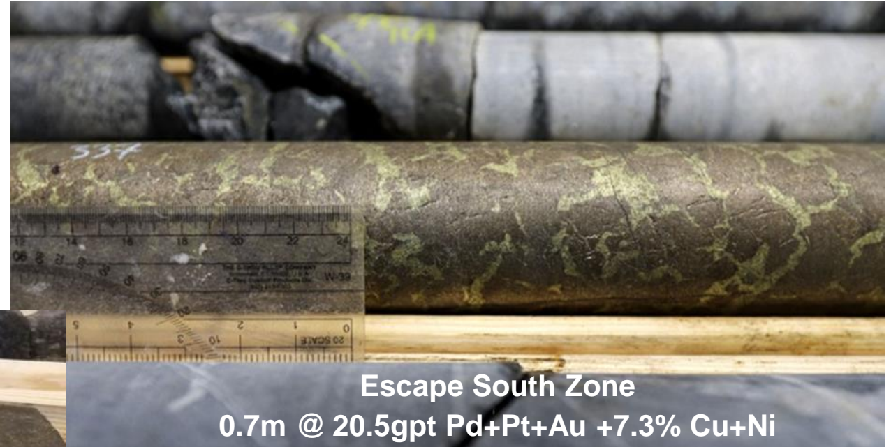
MASSIVE SULPHIDES IN ESCAPE DEPOSIT (HOLE ELR21-041)
